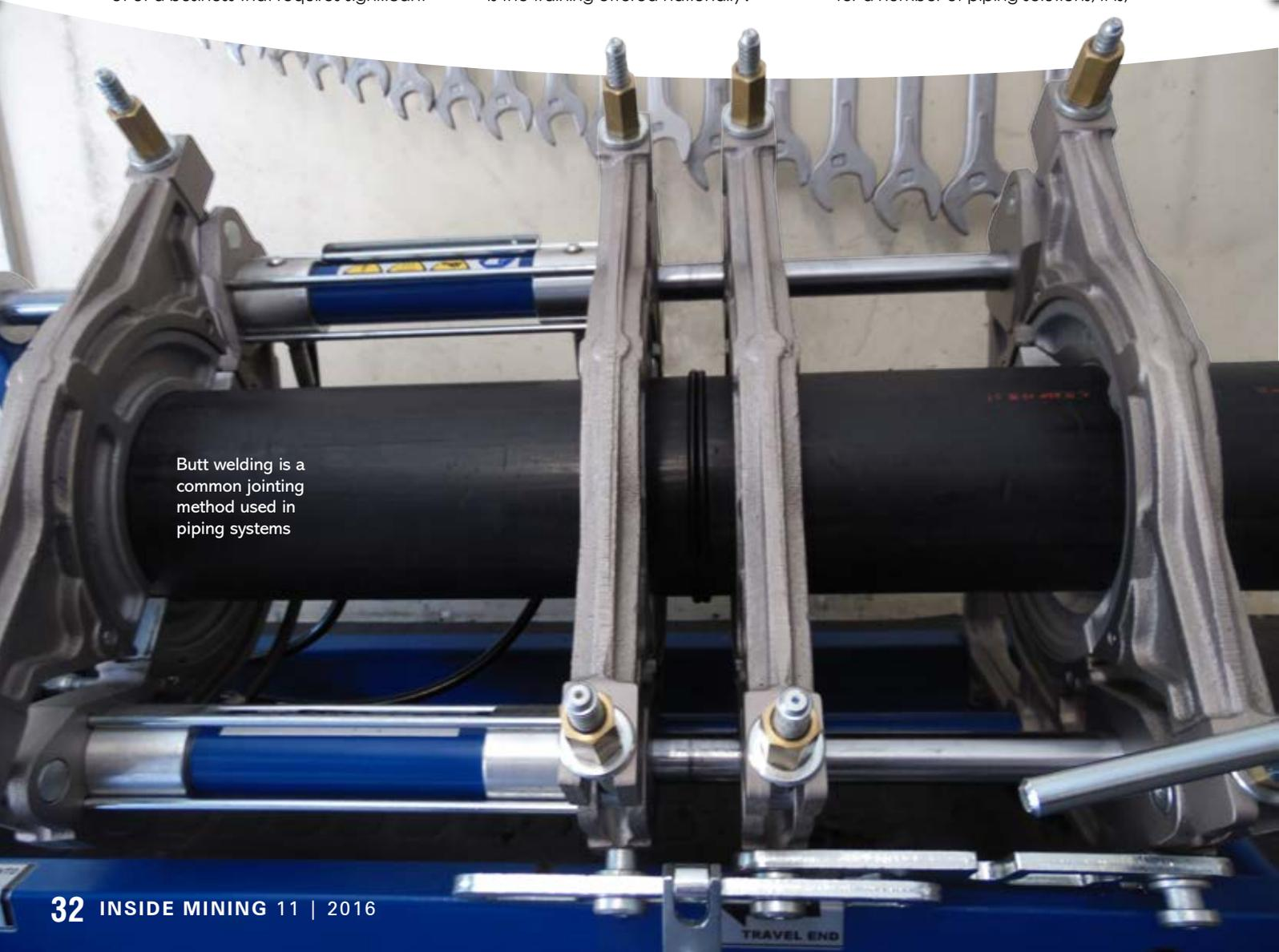
Butt welding is a common jointing method used in piping systems
